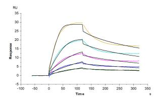
Mouse FcRn, His Tag captured on CM5 Chip via anti-his antibody can bind Trastuzumab with an affinity constant of 1.76 nM as determined in SPR assay (Biacore T200) (QC Test).
